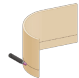
▲ 3-Meter Diameter Arc / Flat Panel Horizontal Alignment Welding
