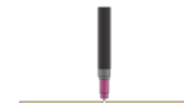
▲ Flat Butt Welding
